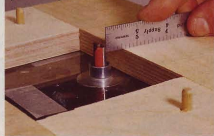
B Adjust the \frac{1}{2} " straight bit so it sticks \frac{3}{16} " above the plate template.
